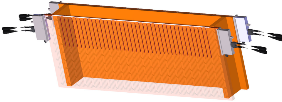
Figure 3: CAD-model of an entire mold with the sensor-equipped copper plates semi-transparent. Each vertical line is an embedded fiber sensor with 70 individual sensor point. The grey boxes are the extra connection boxes where the sensor fibers are connected to harsh-environment cables.
