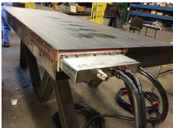
Figure 4: Photograph of the modified copper plate after installation of the sensors, as used in Tata Steel Europe (IJmuiden).
