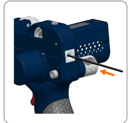
13. Start the compressor. if using bare fibre from the pan. Feed the fibre into the back of the ABF tool so it comes through a short way and reaches the duct you are blowing the fibre into.
