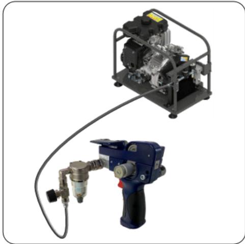
12. Purge the air from the compressor & leave the valves open (see compressor operating guide). Connect the air line, first to the ABF tool, then to the compressor.
