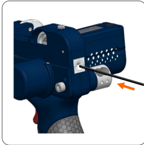
13. Start the compressor. if using bare fibre from the pan. Feed the fibre into the back of the ABF tool so it comes through a short way and reaches the duct you are blowing the fibre into.
