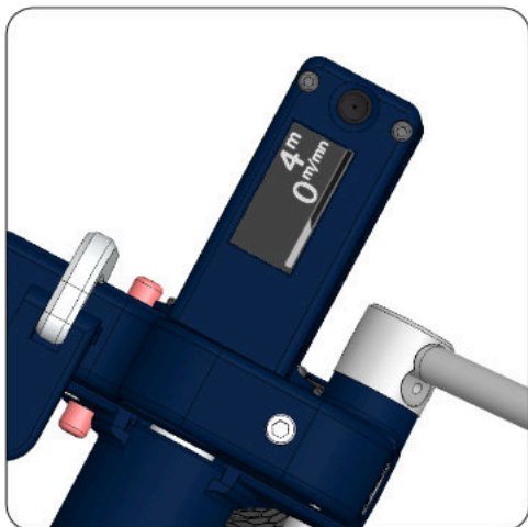
15. The display will show the distance the fibre has travelled and the speed while the fibre is moving.
