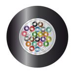
1 Primary coated fiber: Silica, acrylate 2 Filling compound: Thixotropic gel
