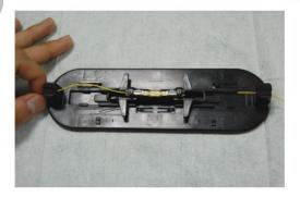
The fibre should be restrained in a light bend
