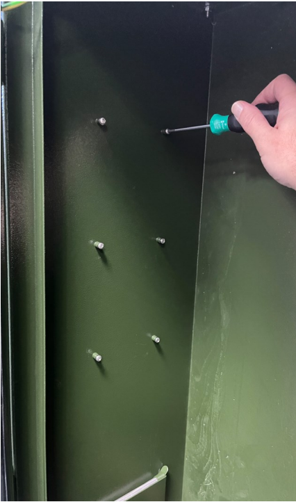
Remove fixing screws from the cabinet
