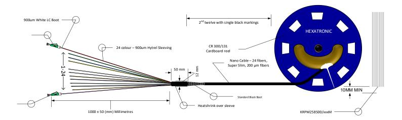
The air blown fibre is designed with durability and performance in mind. A sturdy fibre unit with state of the art fibre blowing performance increases the installation success rate and provides quick and problem free installation.
