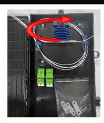
5. Dress the tails away ready to install the connectors into the adapters.
